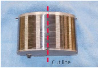
After heat-treating, the wire around the form is cut across the middle on both sides of the form, creating individual archwires.
